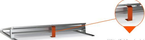
Additional Back Center leg, designed to significantly increase the snow load capacity of each module. Engineered to withstand up to 2,400 Pa of snow and wind loads.
