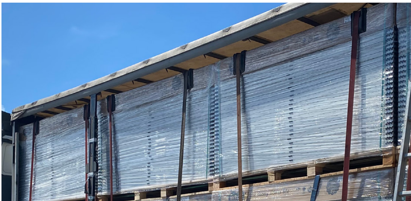
PICTURE 6: Demonstration of the correct installation of cargo security straps and plastic corners.
