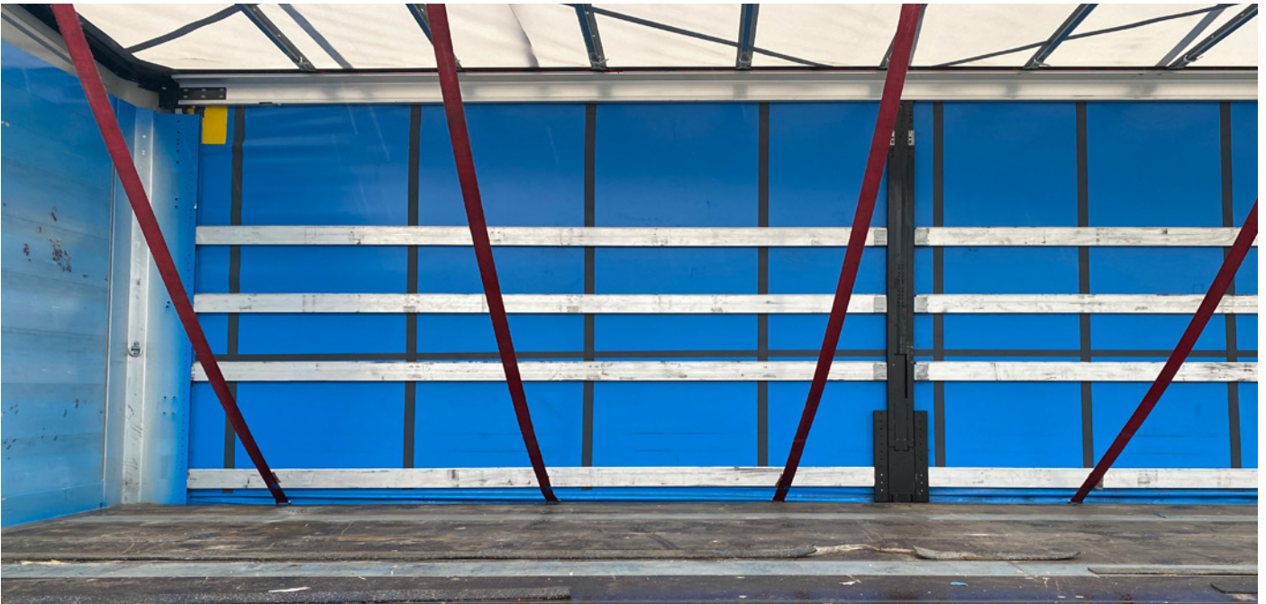
PICTURE 1: Correct placement of the straps before the loading.
