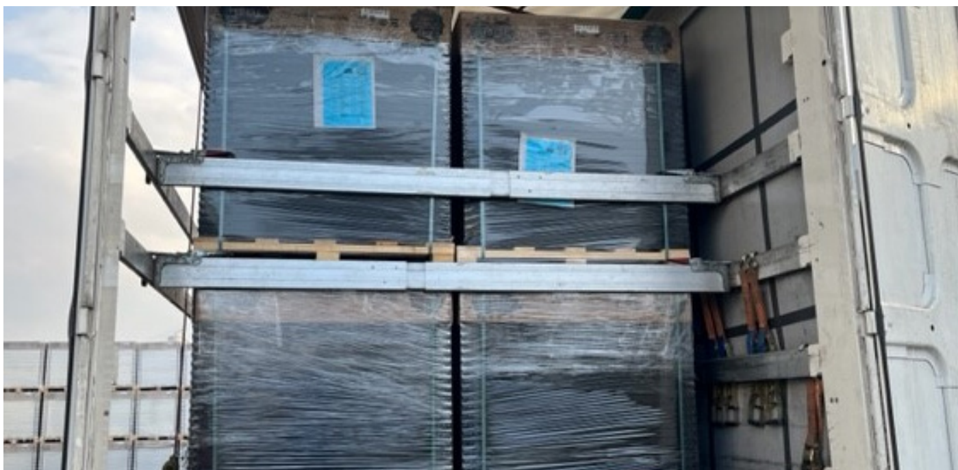
PICTURE 7: Demonstration of using a double intermediate block bar.
