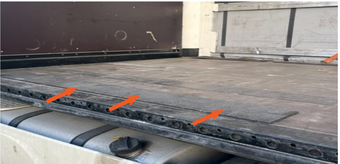
PICTURE 2: Placing the anti-slip rubber.
