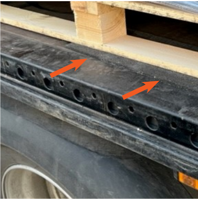
PICTURE 3 and 4: Placing the anti-slip rubber.
