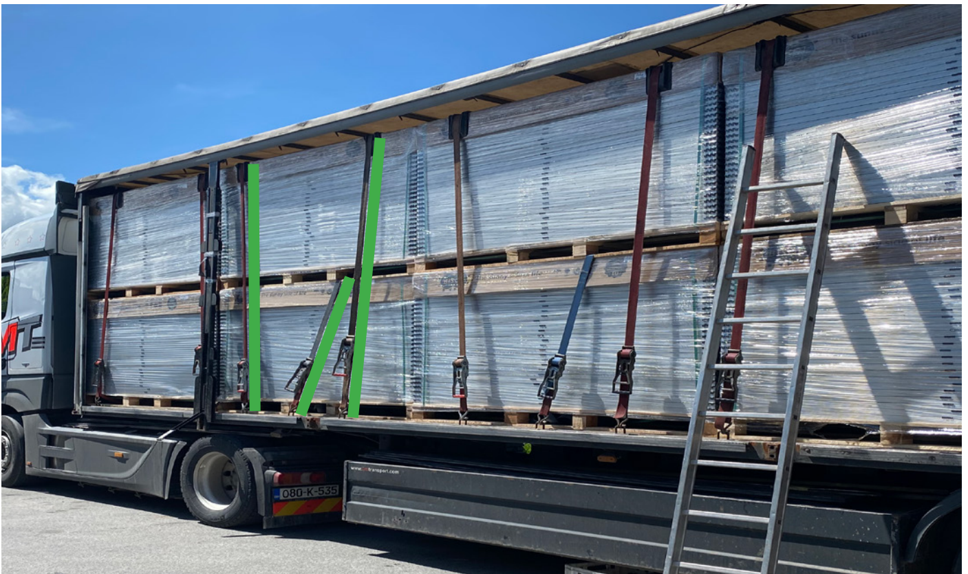
PICTURE 5: Demonstration of proper fastening of cargo security straps (indicated in green).
