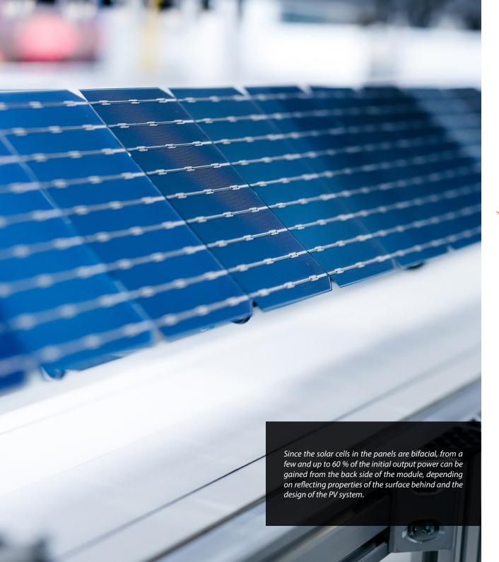
Bifacial Monocrystalline PV Modules with Transparent Backsheet
